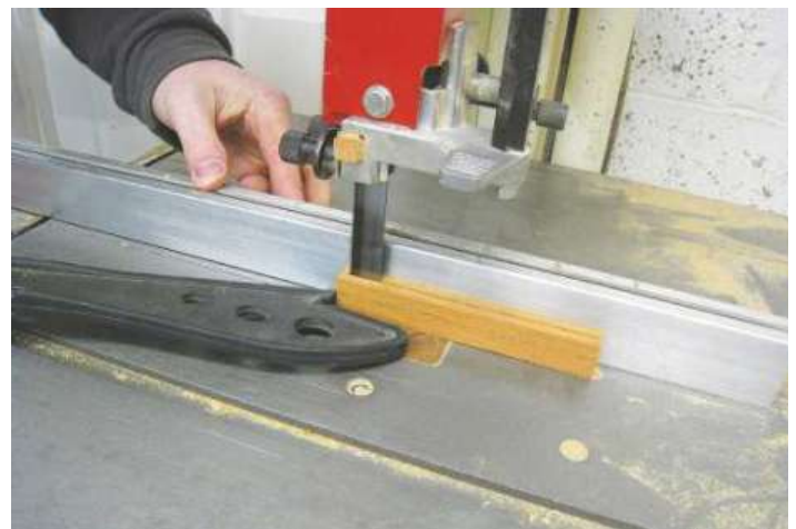
▲ Pic.2 After planing the iroko down to the right thickness, he dimensioned the piece in half on the bandsaw
